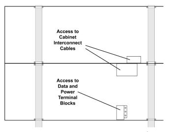
access panel, at the top of the lower cabinet, is the panel covering the lower set of interconnect cabling. Just above this, in the top cabinet, is the panel covering the upper set of interconnect cabling.
